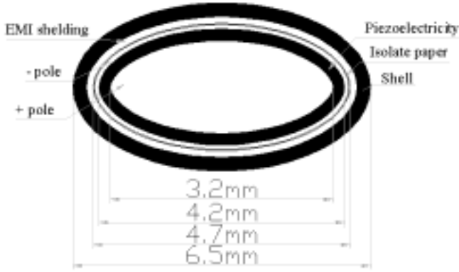
Figure 2. Cross-section of the piezoelectric cable.
