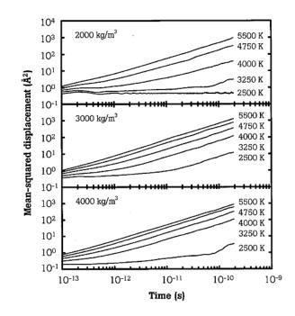
Notice the log-log plot. We see linear behavior in the curves (expected for random-walk diffusion according to a diffusion constant) after some initial time period has passed. There are different regimes in particle diffusion:
