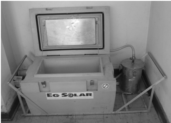
Fig.4. Zeolite-water refrigerator. The adsorber chamber, at right, can be opened, in order to remove the vessel with zeolite
